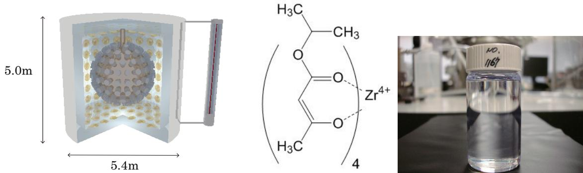
**Figure 1.** The left panel shows the conceptual design of the ZICOS detector. The spherical inner detector will be filled with a liquid scintillator which contains high concentration of  $\text{Zr}(\text{iprac})_4$ . The middle panels shows the chemical structure formula of  $\text{Zr}(\text{iprac})_4$  and the right panel shows a sample liquid scintillator containing 10 wt.% concentration of  $\text{Zr}(\text{iprac})_4$ .
