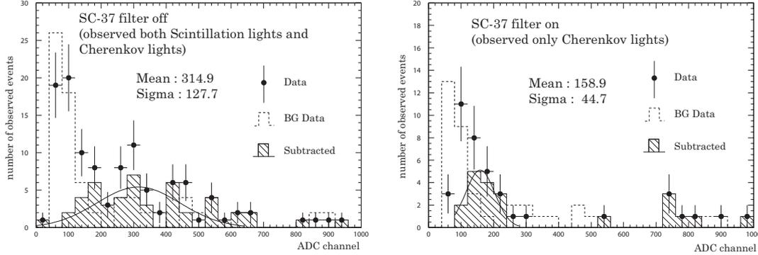
**Figure 3.** The left panel shows the pulse height distribution of no filter, therefore the light includes both scintillation and Cherenkov. The right panel shows only Cherenkov light distribution above 400 nm, which is obtained by using SC-37 UV cut filter.
