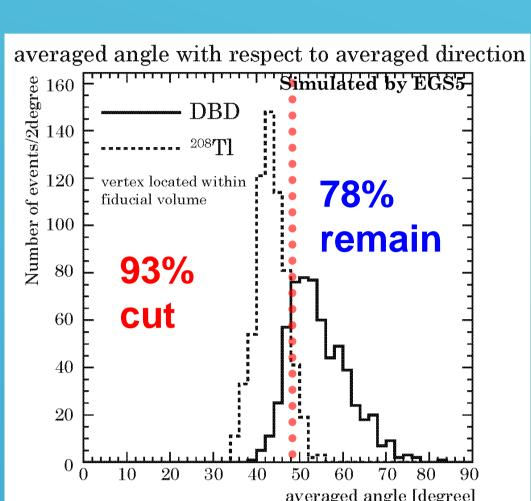
The averaged angle distribution with respect to the averaged direction of single electron has a peak at ~48 degree which is almost same value as Cherenkov angle in Anisole.
