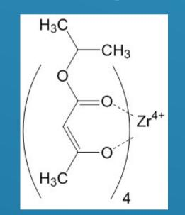
tetrakis (isopropyl acetoacetate) Zirconium: Zr(iPrac)<sub>4</sub> MW: 663.87
