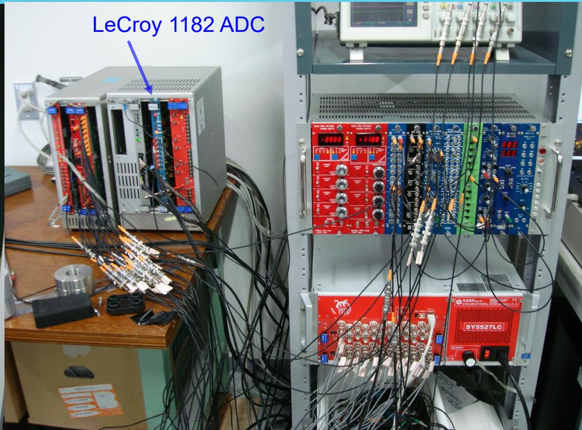
**Problem : MCX cables were connected only half channel due to lager thickness!**
