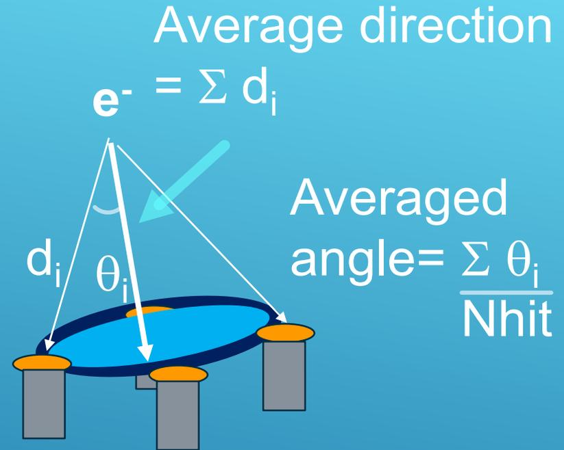
Average angle with respect to averaged direction for single electron seems to have a peak at 48 degree which is almost same as Cherenkov angle.
