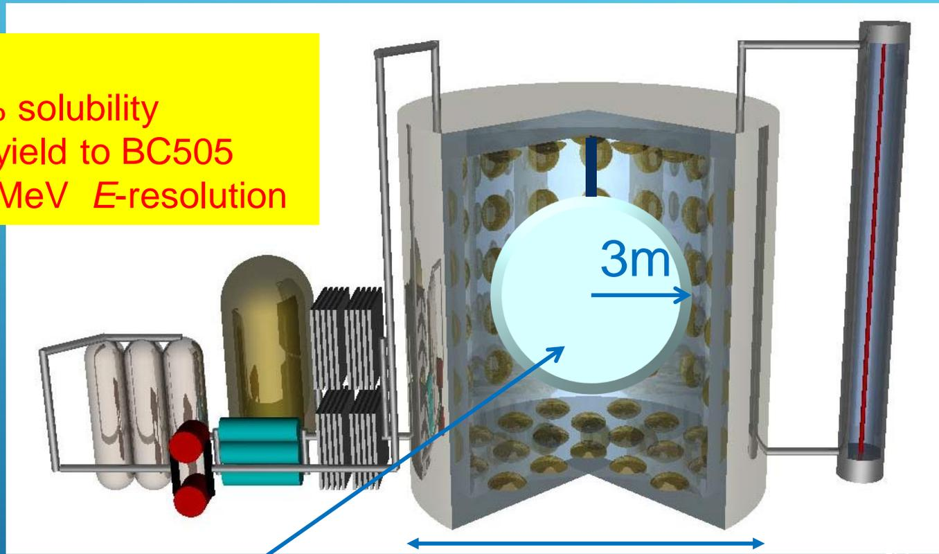
Zirconium loaded 100ton LS
