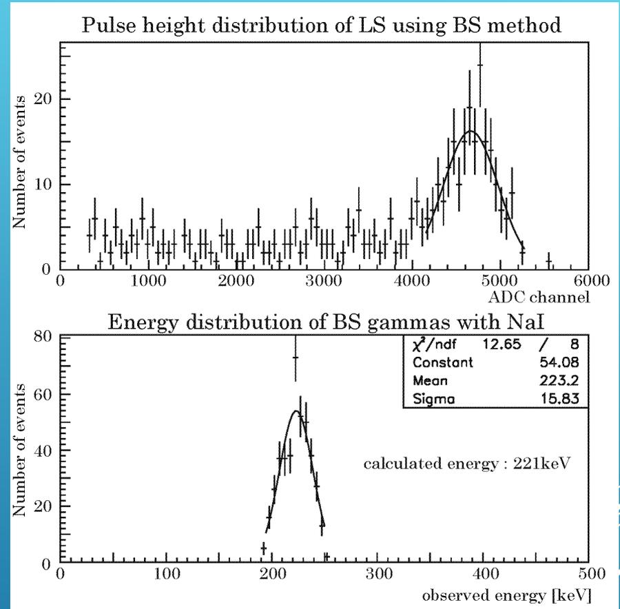
Single peak could be used even in liquid scintillator.
