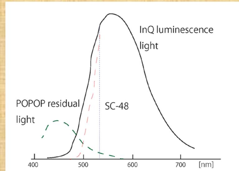
Most of the loss would be POPOP residual lights. It is consistent with the decrease of light yield for  $\text{InQ}_3$  50mg  $\rightarrow$  100mg due to absorption of these light.
