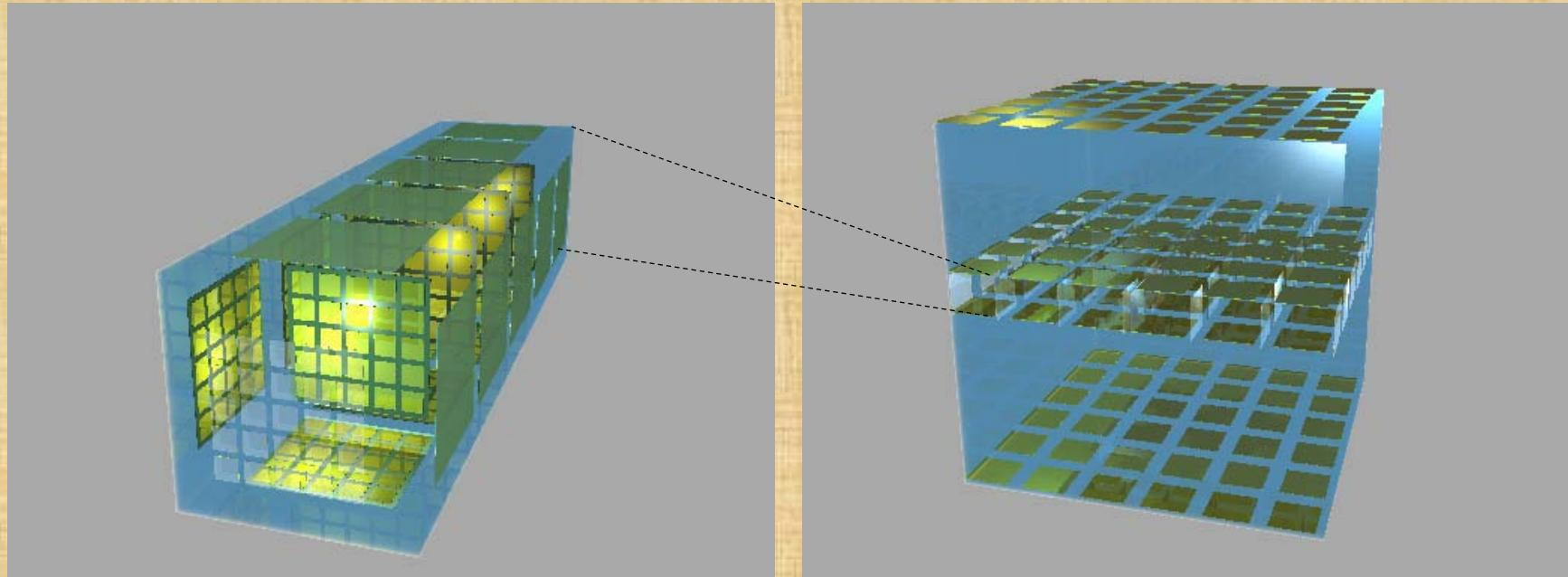
InP cell detector would observe scintillation light from LXe
