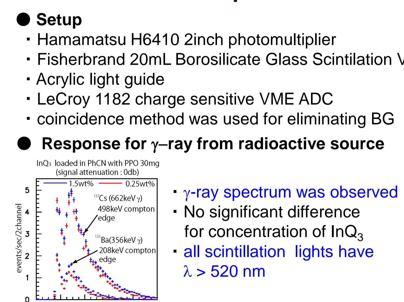
Photo luminescence caused by  $\gamma$ -ray was confirmed
