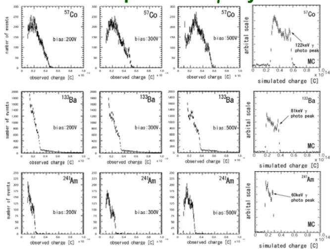
$\gamma$  spectrum obtained by InP detector
