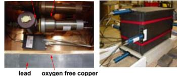
CsI(Tl) scintillator : to detect Bremsstrahlung and other coincidence events with InP detector
