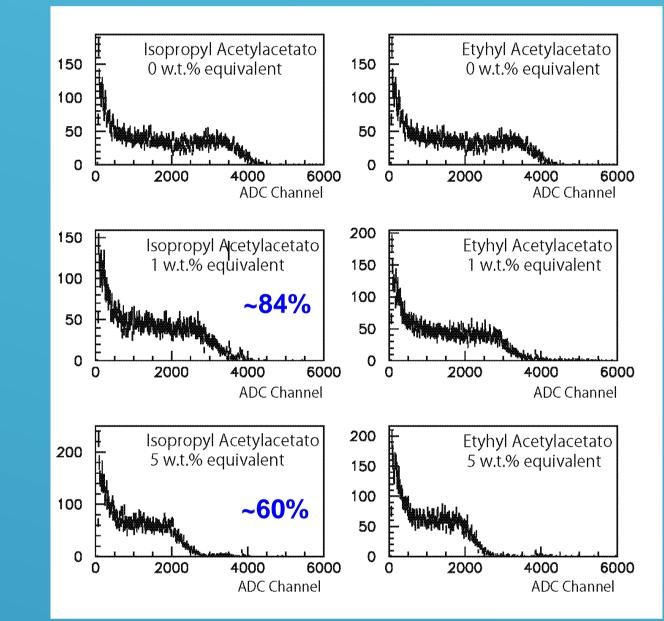
Absorption peaks of  $\beta$ -keto ester ligands were found around at 240nm (not 270nm) even though the aromatic solvent. Scintillation light yield recovers almost double @ 5w.t.%.
