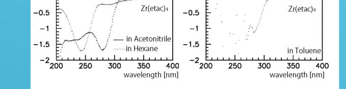
**Confirmed absorption peak moves** 275nm  $\rightarrow$  245nm in Hexane, but in Acetonitrile
