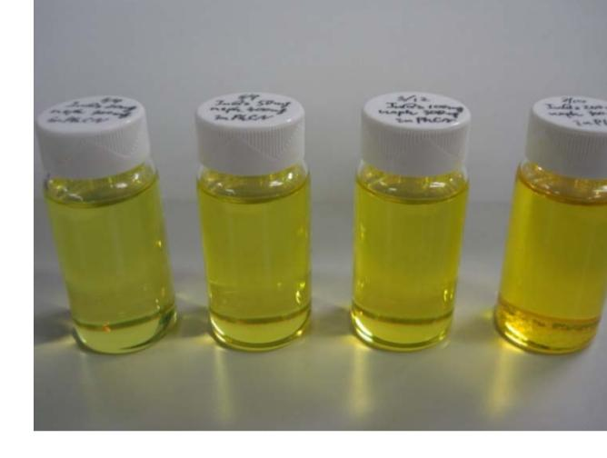
Solvent : Benzonitrile (PhCN: C<sub>6</sub>H<sub>5</sub>CN) density : 1.0g/mL flash point : 75°C Photon emission : 291nm@maximum Solubility of  $\text{InQ}_3$  complex: 2wt% Attenuation length : 66cm (@0.5wt%)
