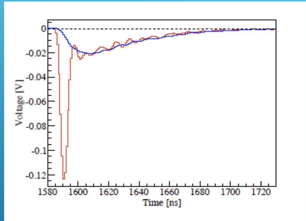
**Cherenkov has a faster peak than scintillation.**
