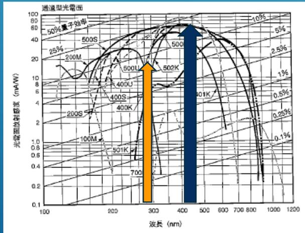
Relative scintillation light yield of **anisole** is 9.8% to **standard cocktail** (due to difference of quantum efficiency of PMT)
