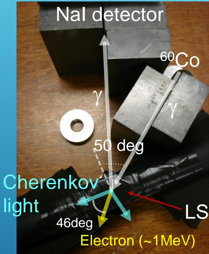
Comparison of light yields between SC-37 filter off and on for anisole only LS using back scattering method.
