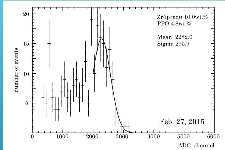
Light yield of  $48.7 \pm 7.1\%$  for BC505, and an energy resolution of  $4.1 \pm 0.6\%$  at 3.35 MeV assuming 40% photo coverage of the photomultiplier are obtained at 10wt.% concentration of  $\text{Zr(iprac)}_4$  with 5 wt.% of PPO and 0.5wt.% of POPOP in anisole.
