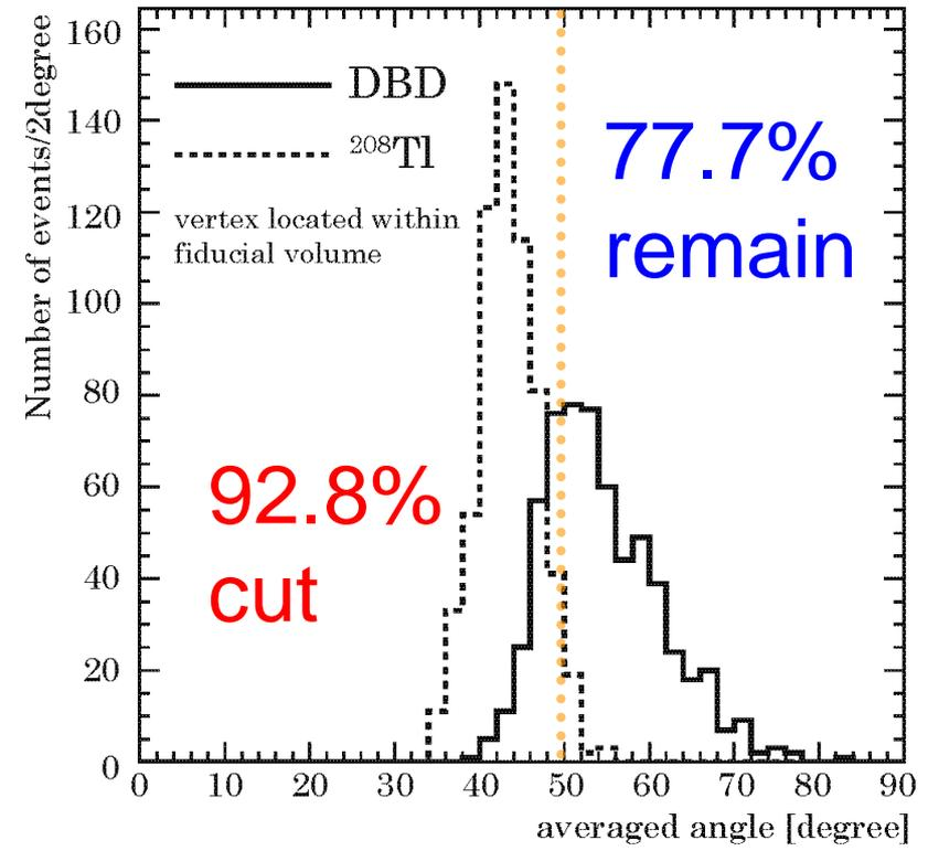
Cherenkov hit pattern can be used for BG reduction.
